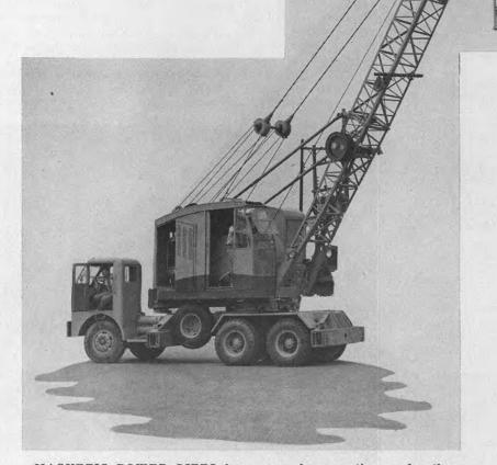
MAGNETIC POWER LIFTS huge crane boom sections under the watchful eye of Jesse A. Floyd, 2417, the magnetic crane operator. The big magnet can raise 5,000 pounds and when the crane is fitted with a hook it can lift 20 tons. Operating the crane tractor here is Stanley D. Brooks, 2417.
